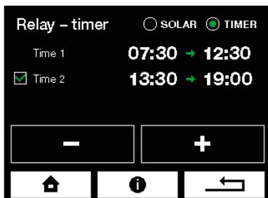
To use this function, in the menu **PROGRAMMABLE RELAY** choose the option **TIMER**. One or two intervals can be set for the activation of the relay. Connect what is to be controlled by the TIMER to the POTENTIAL-FREE relay Timer / Heating.
