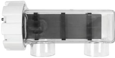
One of the key components of the ASIN AQUA Salt device is the titanium electrode TE-25 with a ruthenium-iridium surface, which enables electrolysis of pool water and chlorine generation.
