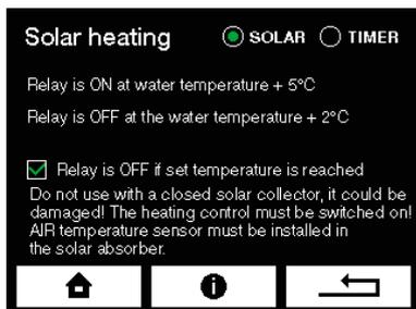
To use this function, in the menu **PROGRAMMABLE RELAY** choose the option **SOLAR**. **Connect the air thermometer to the solar absorber** and to the POTENTIAL-FREE relay TIMER / HEATING connect what is to be controlled by the relay.
