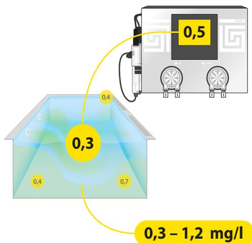
Calibration **is not necessary** if the difference between the photometer measured value and the value shown on the display **is less than 0.2 mg / liter.**
