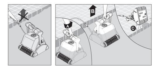
Using the floating cable, bring the Pool Cleaner to the pool's edge.
