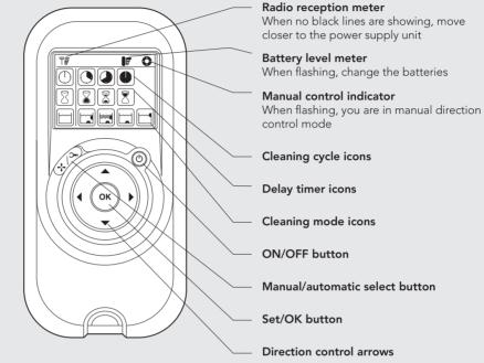
The remote control unit (RCU) offers two operation modes -Automatic mode and manual direction control mode.
