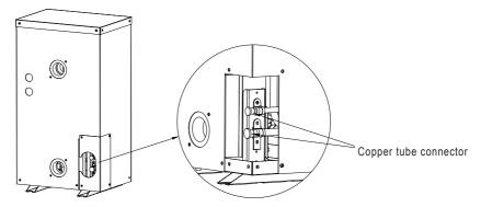
The schematic diagram is for reference only. Please check the water inlet/outlet label on the heat pump while plumbing installation.
