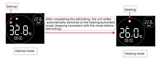
Notes: During the defrosting, mode switch is available. And when switching the mode, the unit won't work under a new mode until defrosting is completed.
