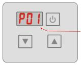
Water inlettemp. Sensor failure
