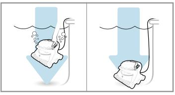
Submerge the cleaner in the pool by gently rocking it back, forth and sideways to help the cleaner purge trapped air and sink to the pool bottom.
