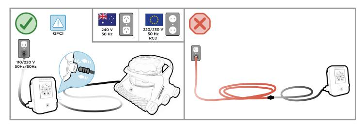
Connect the cleaner cable to the control unit and plug the control unit cord into a protected outlet.
