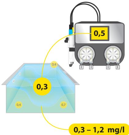
**Do not calibrate the probe until** the water in the pool is thoroughly mixed and **the value on the ASIN AQUA Net display is stable.**
