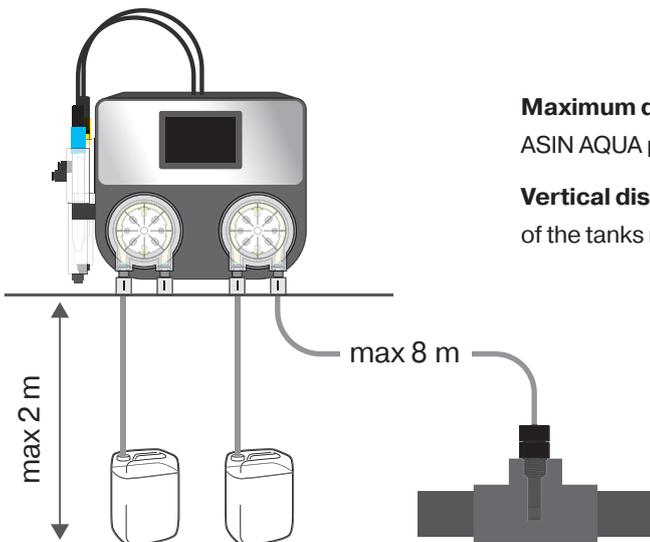
**Maximum distance of injection valves** from peristaltic ASIN AQUA pumps must not exceed **8 m**.
