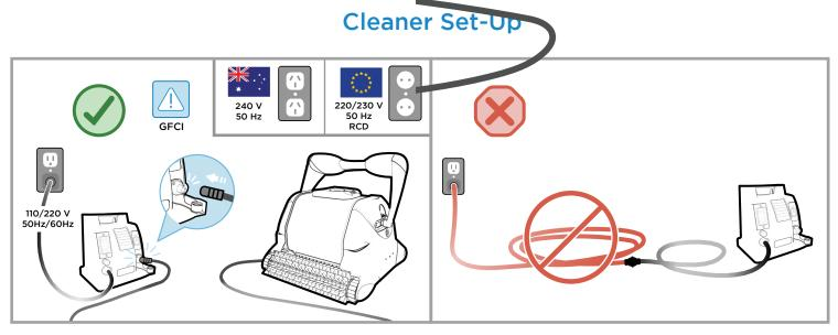
Connect the cleaner cable to the control unit and plug the control unit cord into a protected outlet.
