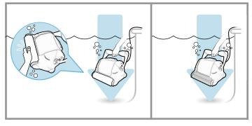
For units with foam rollers, squeeze the foam to allow the roller to get soaked.
