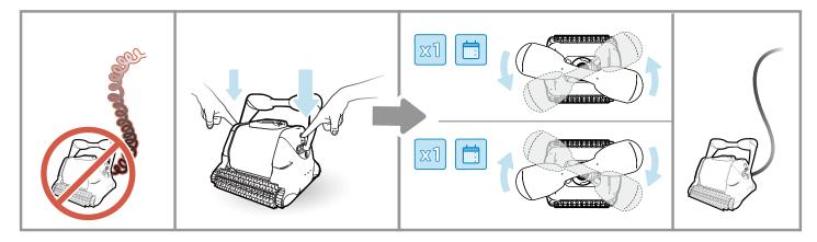
The Aquashark has an adjustable handle. The handle must be locked in a diagonal position in order to ensure optimal cleaning results. The handle has two diagonal positions. Reverse handle positions after each use to minimize cord twisting.
