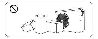
1.4.4. Don't put anything into inlet or outlet, or the efficiency of the heat pump will be reduced or even stopped.
