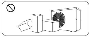
1.4.4. Don't put anything into inlet or outlet, or the efficiency of the heat pump will be reduced or even stopped.
