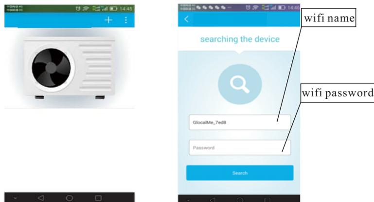
6) Insert default password of the device “123456”, and click “Bar code” to scan the serial number of heat pump which is below the data plate on the side panel of the heat pump.
