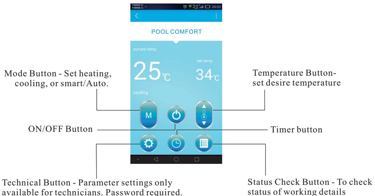
2).How to switch on/off the heat pump.
