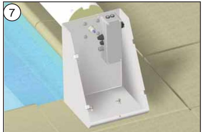
Align the axle with respect to the geometry of the structure. (Measure the diagonals to ensure that the Aquadeck cover is correctly positioned). If installing the wired version, leave a length of 70 cm of cable.
