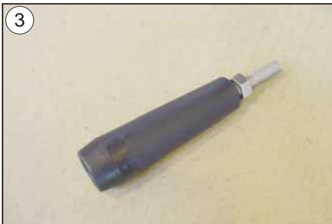
3 Thread the hex socket head cap screw M8x100/28 through the hand-grip and screw the hex nut M8 down to the end of the threading.
