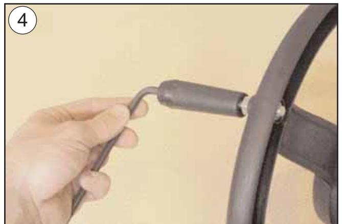
4 Push the hand-grip assembly through the hole in the wheel and fix in position using the second hex nut M8.
