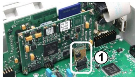
The configuration module is plugged in to a plug socket, making it easy to replace or to plug into another unit.
