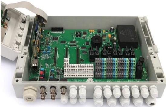
3. Loosen the large cable fitting on the far left.
