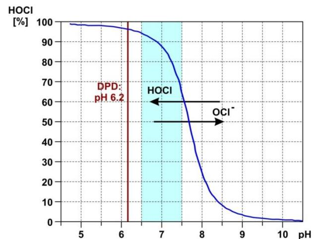
If control measurements are performed using the DPD method, then it is important to know that the DPD measurement is always performed at a pH value of ca. 6.2. That value is attained with an integrated pH buffer in the DPD reagents. Thus, a DPD measurement always measures all free chlorine independently of the actual pH value in the pool. Therefore, a DPD measurement may not be significant for the real disinfection effectiveness, especially, if pH is above ca. 7.5.
