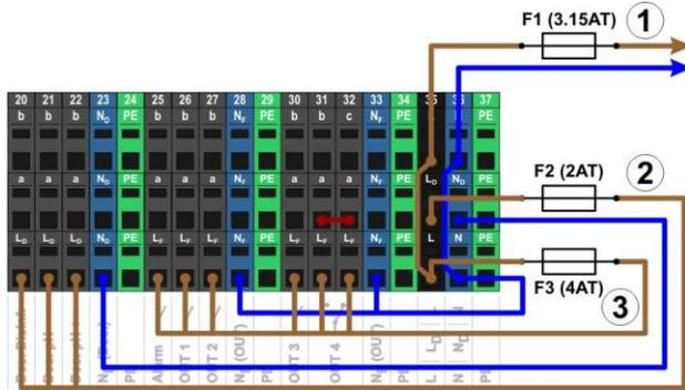
The supply for the Analyt unit as well as for the alarm relay and the add-on functions share a mutual power input (L/N). Phase L for Analyt is run from the input over via fuse F1. Phase L<sub>F</sub> for the alarm relay and the add-on functions is run from the input via fuse F3. Neutral conductors N and N<sub>F</sub> are connected to each other internally.
