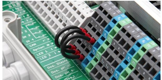
Wire bridges in the terminal box from phase L<sub>D</sub> to the dosage outputs' centre relay contact a
