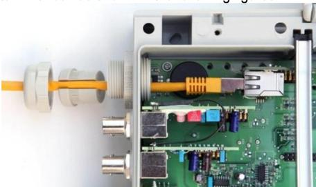
5. Next, run the cable through the cable fitting's cover and through the fitting itself.
