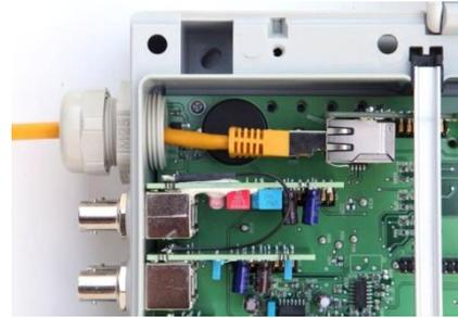
9. Screw the cable fitting tight again in order to obtain a reliable seal.
