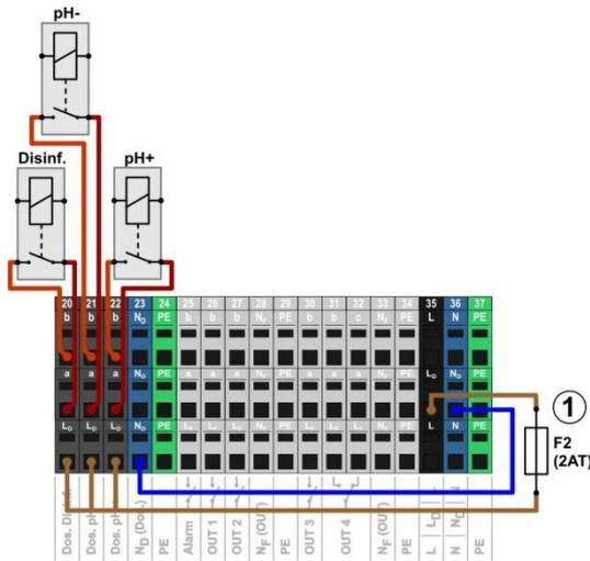
1 Fuse 2AT for the 230V~ Phase L<sub>D</sub> for supplying dosing outlets
