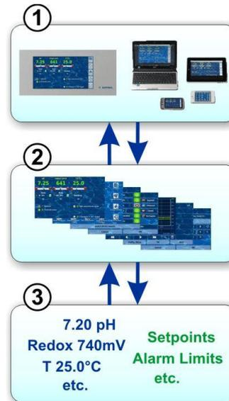
Analyt WebGUI facilitates complete and entirely transparent remote access from a local network (TCP/IP, Ethernet) or from the Internet. Transparent remote access means that the user interface looks exactly like it does locally on the Analyt unit and is operated identically.
