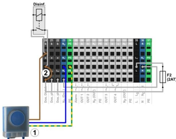
1 Standard dosing pump 230V~ (peristaltic pump)
