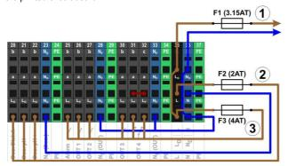
The supply for the PoolManager® unit as well as for the alarm relay and the add-on functions share a mutual power input (L/N). Phase L for PoolManager® is run from the input over via fuse F1. Phase LF for the alarm relay and the add-on functions is run from the input via fuse F3. Neutral conductors N and NF are connected to each other internally.
