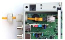
8. Press the rubber seal into the cable fitting
