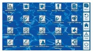
Display and operation are realised on a large TFT colour display with touchscreen. The function shown can be executed with the simple tap of a finger on the corresponding area on the screen. Each tap on the touchscreen is confirmed with a signal tone.
