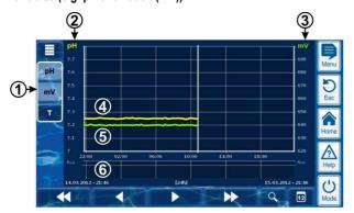
Selection keys for showing one or two measured variables Pressing a key activates or deactivates display of the respective measured variable.
