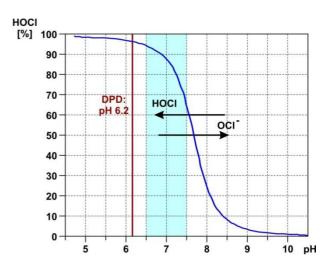
If control measurements are performed using the DPD method, then it is important to know that the DPD measurement is always performed at a pH value of ca. 6.2. That value is attained with an integrated pH buffer in the DPD reagents. Thus, a DPD measurement always measures all free chlorine independently of the actual pH value in the pool. Therefore, a DPD measurement may not be significant for the real disinfection effectiveness, especially, if pH is above ca. 7.5.
