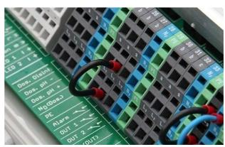
Wire bridge in the terminal box from phase L<sub>F</sub> to centre relay contact a
