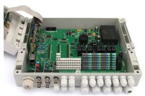
3. Loosen the large cable fitting on the far left.
