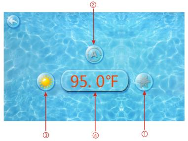
Click the refrigeration mode button ①, automatic mode button② or heating mode button ③then you can select the corresponding mode.
