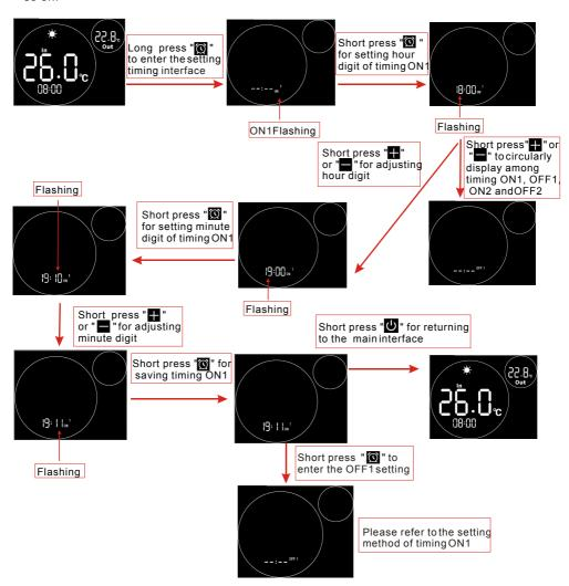
Notes: If there is no operation for 20 s, the system will automatically memorize user's setting, and return to the main interface; If the timing symbol and entire time digits flash at the same time, click " " for returning to the main interface.
