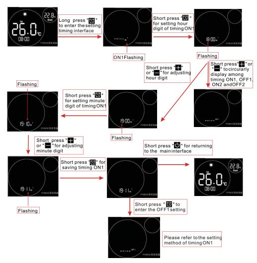
Notes: If there is no operation for 20 s, the system will automatically memorize user's setting, and return to the main interface; If the timing symbol and entire time digits flash at the same time, click """ for returning to the main interface.
