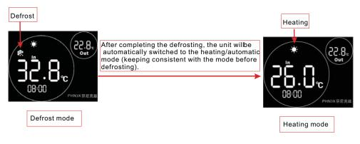
Notes: During the defrosting, mode switch is available. And when switching the mode, the unit won't work under a new mode until defrosting is completed.
